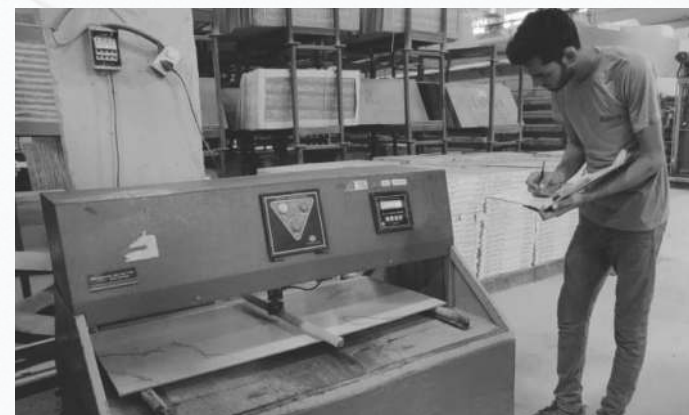
Tile Breaking Strength Check (MOR)
